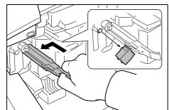
11 With the main charger pulled out about 5 cm (2 inches), remove the grid cleaner. Then push the main charger back in fully, applying pressure in the direction shown by the arrow so that the main charger is in its designated position.
